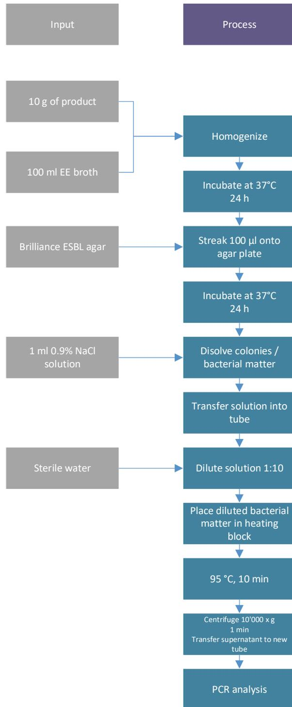
Figure 6: Process flow sheet ST 131 identification from food samples.
